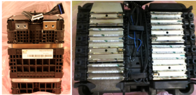
Figure 1: Complete A123 Power System's start-stop battery module (left), and view underneath the top cover (right).
